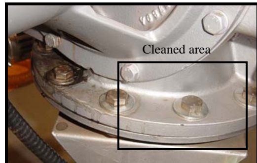
Coffee powder easily melted and blown to floor where it can be recovered with vacuum. Unlike compressed air broadcasting of powders is not a problem.
