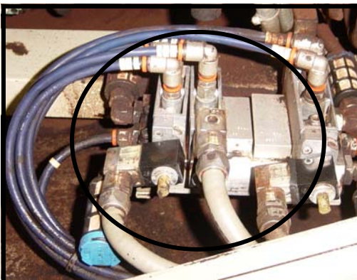
Indicated areas blown clean using long lance. Note absence of any water under the terminal blocks in the picture to the left.
