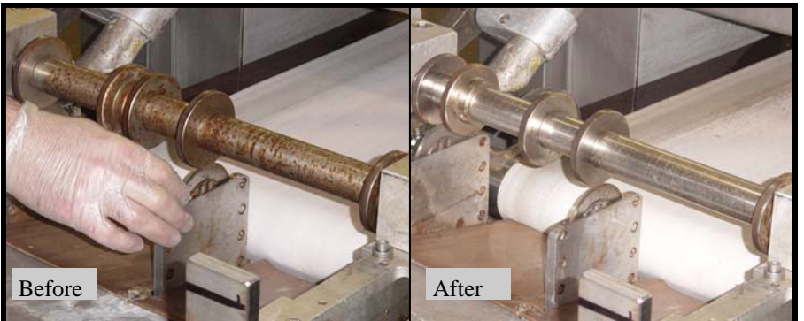
Fig 4 and 5 - Packaging cutters had a buildup of surface rust and corrosion that was providing refuge for bacteria. Normal sanitation was ineffective in removing this but UltraVapor restored the slicer and left it sanitized and dry.
